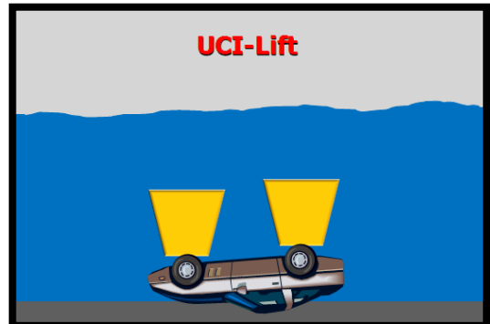
Attach a UCI-VLS bag to each axle on one side with the 4-ft. rigging chain
